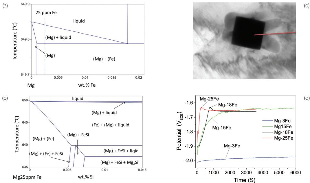
**FIGURE 1.** (a) The solidification interval of Mg-Fe phase diagram, (b) the ternary Mg-Fe-Si phase diagram at constant 25 ppm Fe showing an enlarged solidification interval, (c) TEM images of a typical Fe-rich particle and (d) open circuit potential as a function of immersion time, revealing the surface film breakdown potential that is controlled by the cathodic reaction at Fe-rich particle.
