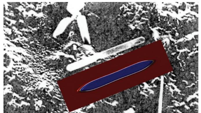
FIGURE 2. Comparison of the morphology of  $Al_{13}Fe_4$  needle crystals. Experimental micrograph is for such needles growing in an Al matrix from Ref [2]. Inset is the simulation using the methodology reported here.
