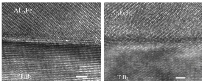
**FIGURE 1.** High resolution TEM images showing the direct evidence of Fe-IMCs nucleated on the modified  $\text{TiB}_2$  particles (a)  $\text{Al}_{13}\text{Fe}_4$ / $\text{TiB}_2$ , and (b)  $\delta\text{-Al}_4\text{FeSi}_2$ / $\text{TiB}_2$ .
