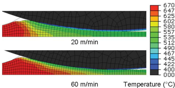
FIGURE 1. Modelled temperature distributions resulted from different casting speeds.
