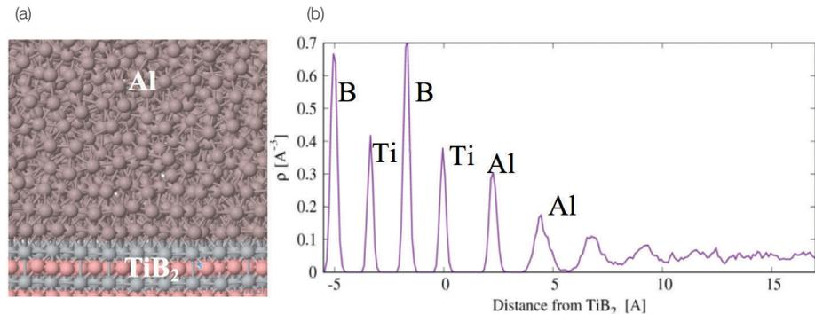
**FIGURE 2.** (a) The Al<sub>3</sub>Ti layer at 1400 K as viewed along the z axis. Atoms are coloured as follows: Blue: ordered Al, Orange: ordered Ti, Pink: disordered Al, Grey: disordered Ti. (b) The density profile of Al<sub>3</sub>Ti at 1400 K
