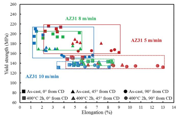
**FIGURE 2.** The tensile properties of the Mg alloy strip produced with different casting speeds.
