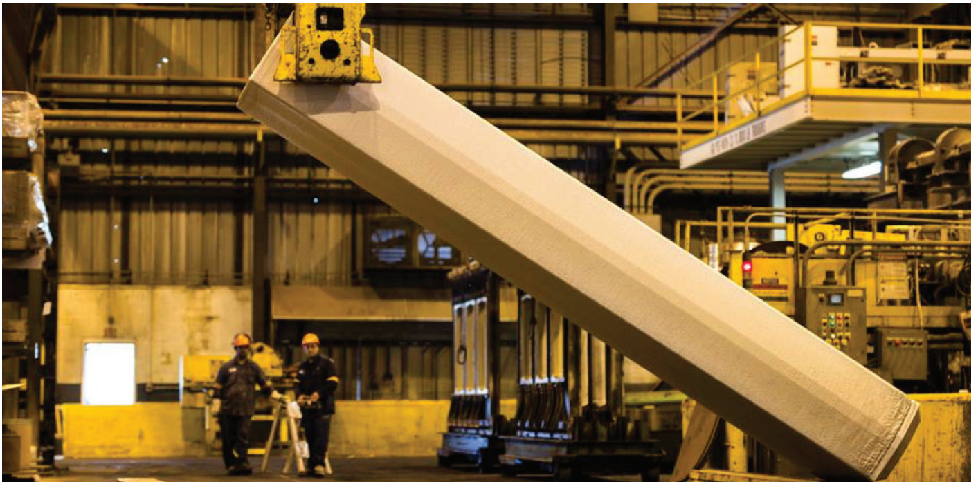
FIGURE 1. Typical large-scale slab casting of aluminium for aerospace applications.
