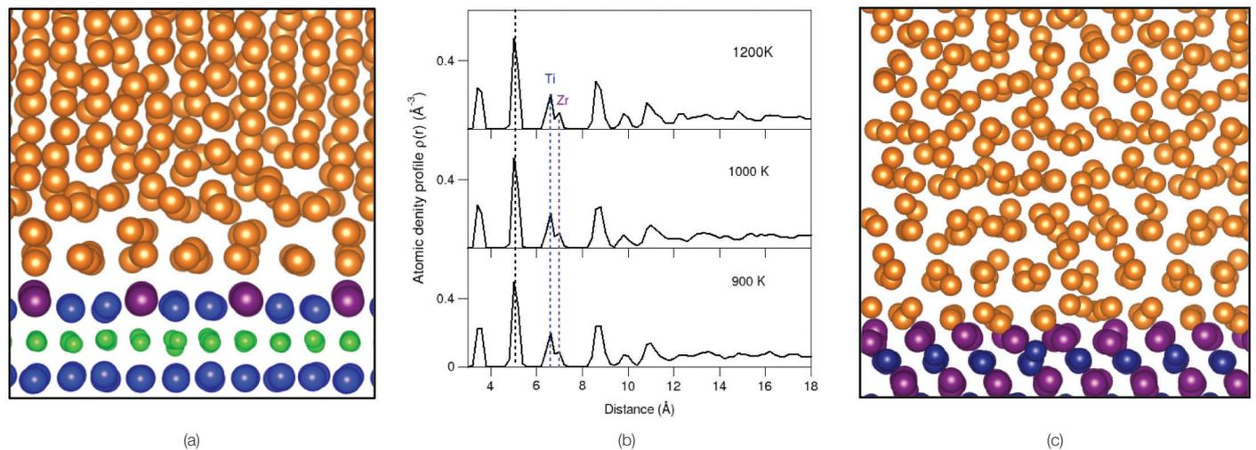
**FIGURE 1.** (a) Snapshot at 1000 K and (b) density profiles of liquid Al/TiB<sub>2</sub>(0001) with ZrTi<sub>2</sub> 2DC (green, Ti; blue, Ti; purple, Zr), and (c) snapshot of liquid Mg/MgO(111) at 1000 K (dark blue, Mg; purple, O). In both cases the substrate surface becomes atomically rough.
