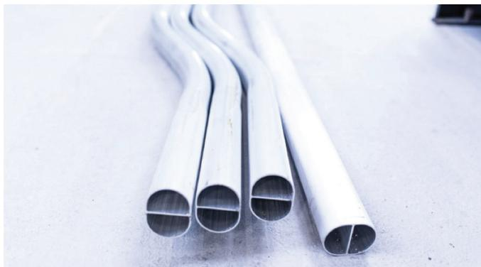
**FIGURE 3.** CAAHS 3D extruded tubes bent in 2017.
